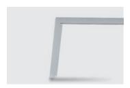
SINGLE CABLE MANAGEMENT FROM THE LEG FRAME 1 mm thick folded sheet metal column in "C" shape. 31,5 x 38,2 mm and 584 mm height. Fixation to leg by pressure.
