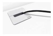
SQUARE DESK GROMMETS ABS tap of 94 x 94 mm and polished finish. Polypropylene piece Ø 80 mm inner. Height 25 mm (2 mm over top).
