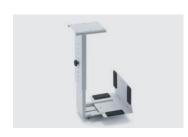
ADJUSTABLE CPU CABINET Support folded metal sheet, 2 mm thick. Adjustable height and width to suit different dimensions. Screwed to desk top. Flexible polyurethane protections to prevent vibration and to ensure an optimal fit.
